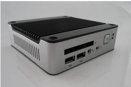
This device is a mini PC that is simply connected to the stores internet via an Ethernet cable that plugs from the device into an available internet port within the store. The unit is completely silent and sized approx. 11cm square it fits easily into most communications cabinets
